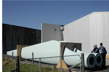
Wind turbine blades for the *Windflow* two-bladed turbine, constructed in Christchurch and operating since 2004.
