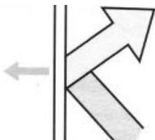
**Reflective insulation reflects radiant heat.**
