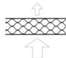
**Bulk insulation traps air in still layers, reducing heat conduction and convection.**
