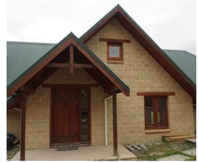
**Alexandra example of thermal mass** provided by earth brick walls inside and out, with a central insulation layer, creating a thick wall. Window openings are timber lined and windows are double glazed, in timber frames.
